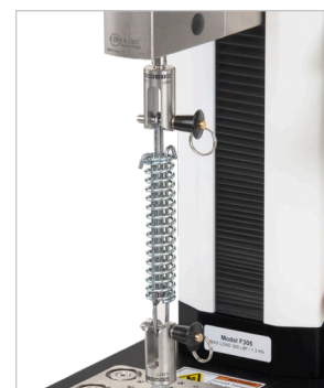
Tension spring testing
