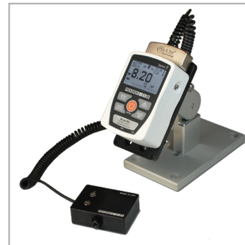
The M3I is shown mounted to an optional AC1008 tabletop stand with Series R03 force sensor
