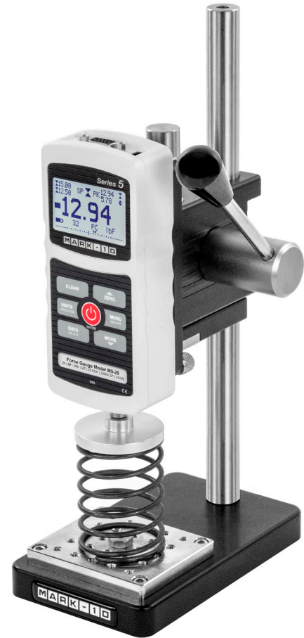
The ES05 is shown in a spring compression test, with Series 5 digital force gauge and 2" compression plate
