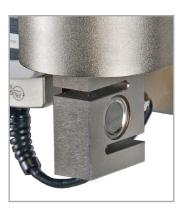
Series R01 sensor with shortened cable is shown mounted to a legacy ESM1500LC test stand.\*
