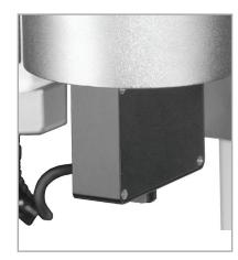
Series R03 sensor with shortened cable is shown mounted to a legacy ESM1500LC test stand.\*
