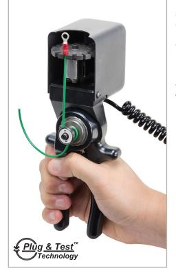
The MR06-200 wire crimp pull sensor is a hand-operated solution for measuring wire crimp pull-off forces. The ergonomic handles and convenient tensioning mechanism make field measurements a breeze for applications up to 200 IbF (1,000 N). Squeeze the handles together to increase tension on the sample until a break occurs. The peak force is recorded by the indicator.
