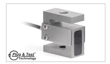
Series R07 force sensors measure tension and compression force, and are designed for use with Models F755, F755S, F1505, and F1505S test frames. Capacities available from 50 to 1,500 lbF [250 N to 7.5 kN]. Also compatible with Mark-10 indicators (sold separately) through unique Plug & Test® technology. Includes a certificate of calibration with data.
