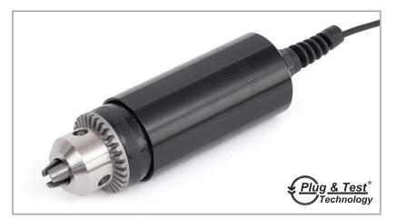
Series R50 smart sensors measure bi-directional torque for a wide variety of applications across virtually all industries. Contain a Jacobs chuck for up to 0.5 in [12.7 mm] diameter samples, bits, or fixtures. The sensors can be used as hand held devices, or mounted to a test stand. Capacities available from 10 ozFin to 100 lbFin [7 to 1150 Ncm]. Compatible with Mark-10 indicators (sold separately) through unique Plug & Test\* technology. Includes a certificate of calibration with data.
