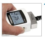
The Plug & Test\* connector locks into the receptacle in the indicator when fully inserted. Dual buttons on the indicator housing release the connector for easy removal. Gold plated spring contacts ensure long lasting and reliable connection.
