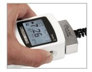
The Plug & Test® connector locks into the receptacle in the indicator when fully inserted. Dual buttons on the indicator housing release the connector for easy removal. Gold plated spring contacts ensure long lasting and reliable connection.
