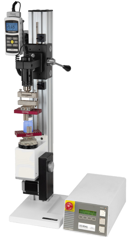
▲ Model TSTM-DC is shown in a cap torque test, with a Series R50 torque sensor, M51 force/torque indicator, G1023 universal closure grip, and G1053 cap grip
