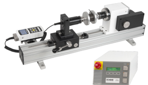
▲ Model TSTMH-DC is shown in a torsion spring test, with a Series R50 torque sensor and M51 force/torque indicator
