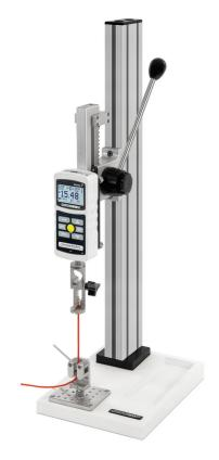
The TSB100 is shown with a Series 7 force gauge, G1001 wire terminal grip, and G1002 dual roller grip.
