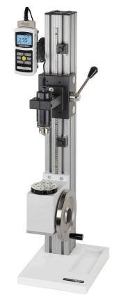
The TST is shown with a Series R50 torque sensor and Model M5I force/torque indicator
