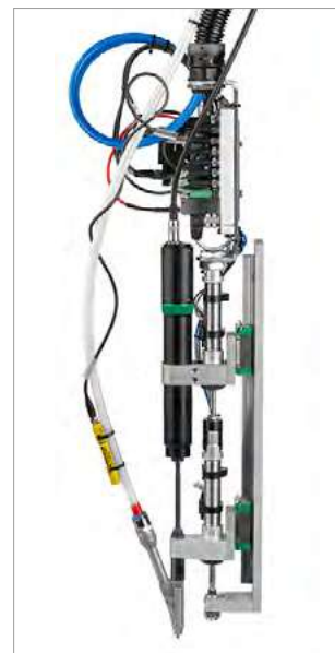
Application example of nutrunner motor on fastening slide
