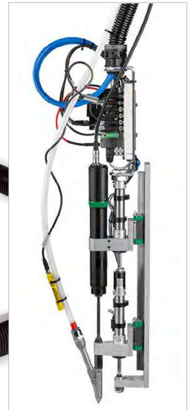
Fastening slide with electric nutrunner motor eTensil.
