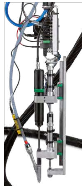
Application example of nutrunner motor on fastening slide
