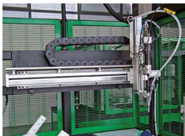
Nutrunner motor operating on Cartesian x, y axes
