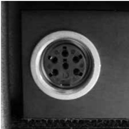
*Load Cell Sensor Plug Connector*
