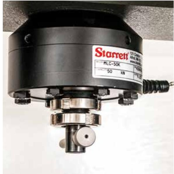
*Clevis adapter attached to load cell sensor*
