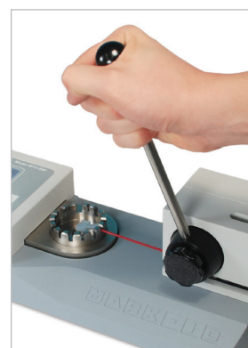
▲ Ergonomic lever easily applies force and releases the sample.
